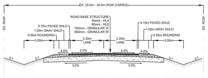
ALTERNATIVE 3 - IMPROVED PAVEMENT STRUCTURE - MINOR LANE WIDENING - WITHIN EXISTING ROW
