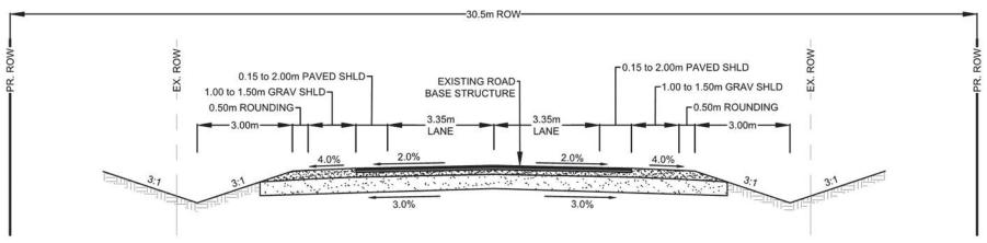
NOTE: WIDTH OF SHOULDER TO BE DETERMINED AS PART OF CONSIDERATION OF DESIGN ALTERNATIVES AND PURPOSE OF SHOULDER (e.g., TO REDUCE MAINTENANCE, TO IMPROVE SAFETY, TO PROVIDE UNBUFFERED BICYCLE ACCESSIBLE SHOULDER OR TO PROVIDE BUFFERED BICYCLE ACCESSIBLE SHOULDER).
