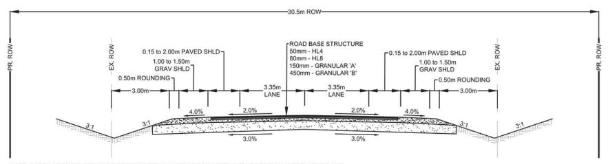
NOTE: WIDTH OF SHOULDER TO BE DETERMINED AS PART OF CONSIDERATION OF DESIGN ALTERNATIVES AND PURPOSE OF SHOULDER (e.g., TO REDUCE MAINTENANCE, TO IMPROVE SAFETY, TO PROVIDE UNBUFFERED BICYCLE ACCESSIBLE SHOULDER OR TO PROVIDE BUFFERED BICYCLE ACCESSIBLE SHOULDER).
