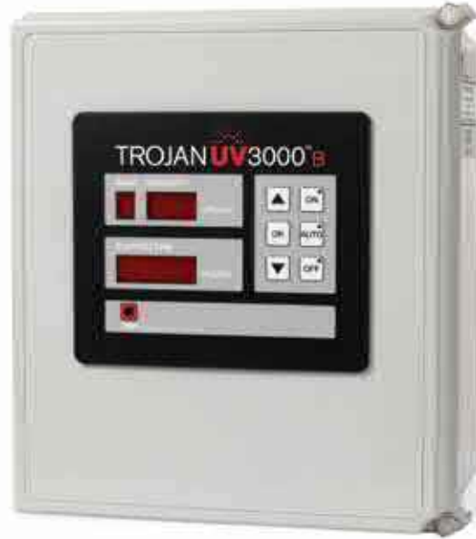
The System Control Center of the TrojanUV3000™B monitors lamp hours and uses a submerged UV Sensor to feed accurate data on UV intensity for at-a-glance system status. The SCC also allows flow pacing to minimize operating and maintenance costs by turning banks on and off based on flow requirements
