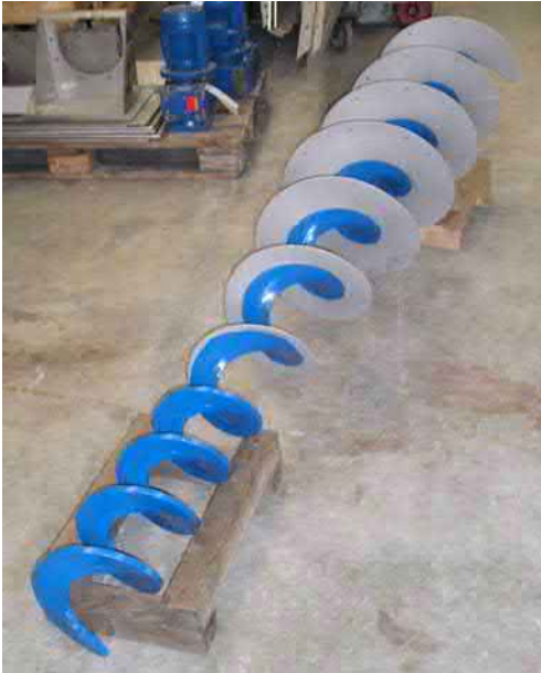
Figure 2 – Continuous ID spiral flight is painted blue. Added flight height in the cone and basket is highlighted in gray.
