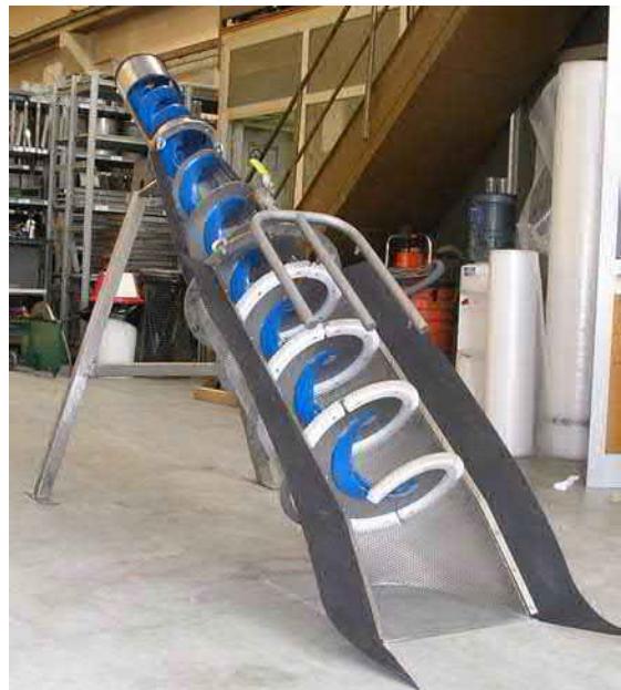
Figure 4 – Cutaway view of a WesTech unit and spiral.
